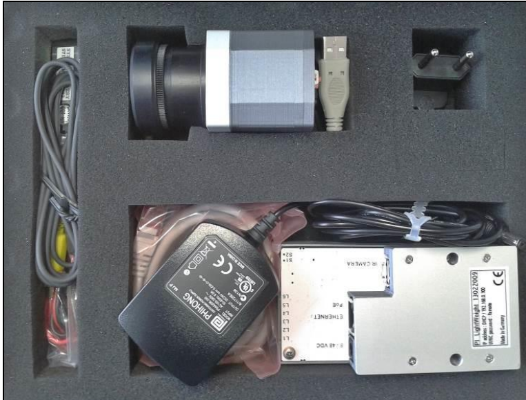
Arrangement of the PI LightWeight kit inside the camera case
