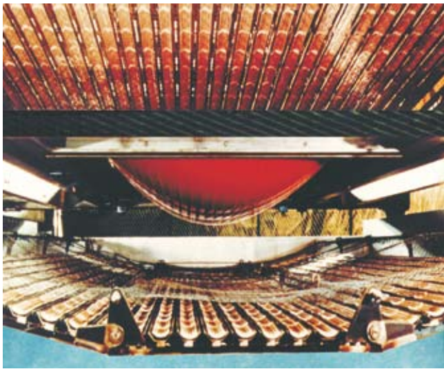
Figure 7: Thermoforming plant for boat hulls
