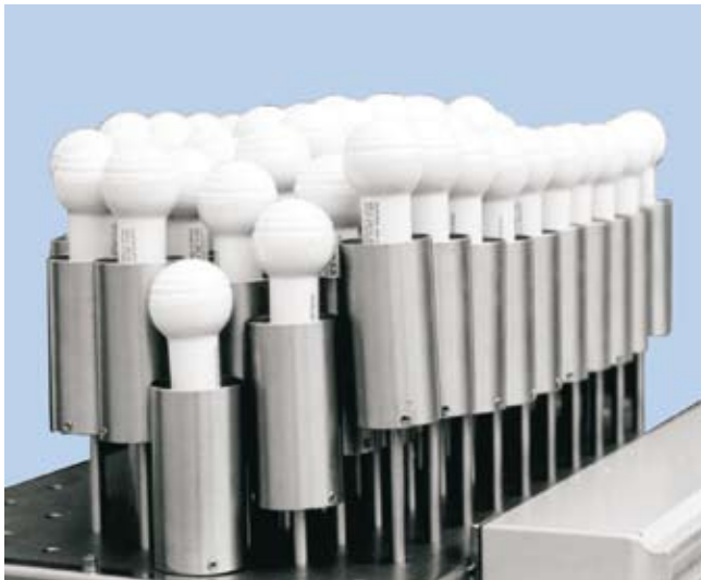
Figure 8: 3-D heating panel for laminating door trims
