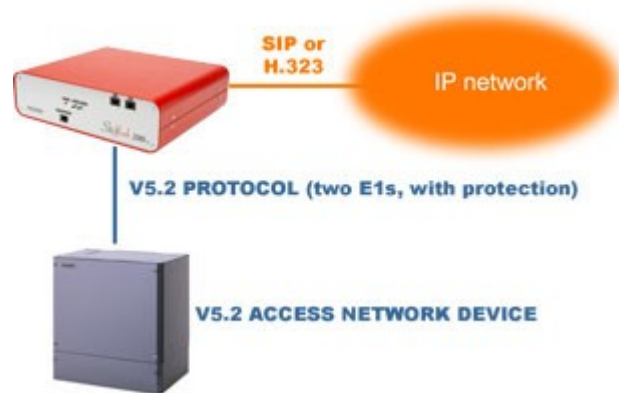
Stillink 200 V5.2 VoIP Access Gateway with protection protocol
