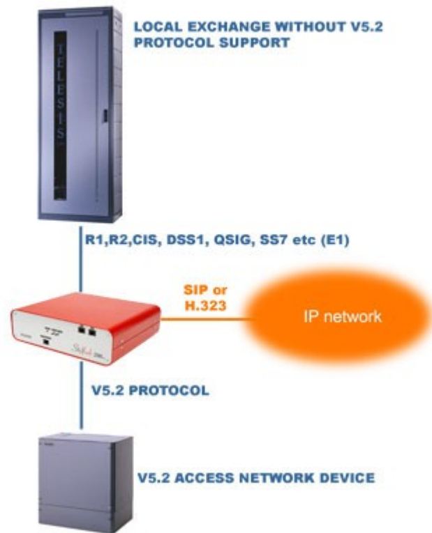
Stillink 200 V5.2 VoIP Access Gateway with PSTN redundancy
