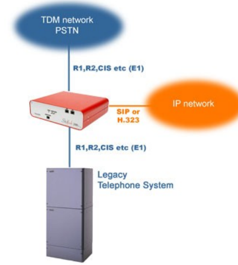
Stillink 200 digital CAS-VoIP gateway with PSTN by-pass capability
