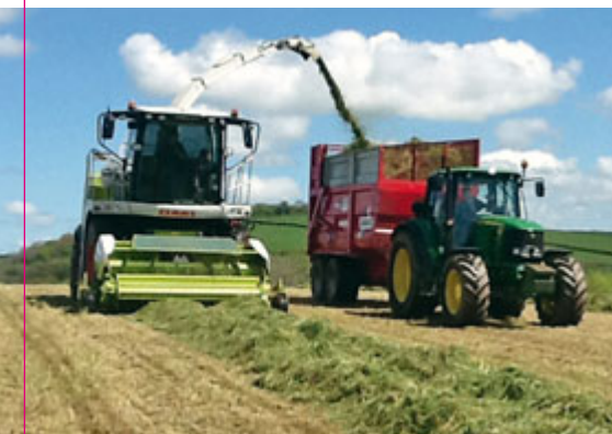
IDM Services' Claas Jaguar 940 forager is equipped with yield metering, telemetry and a tyre inflation system for harvesting grass, maize and whole-crop cereals.
