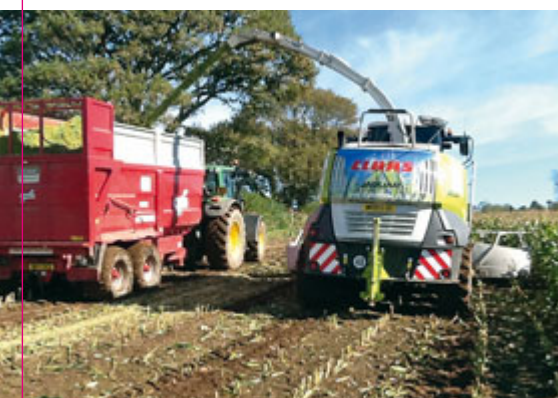
One of IDM's 14t trailers is equipped with a strain-gauge weigher. This provides data to help calibrate the forager's yield monitor.
