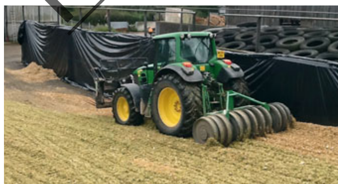
The 3m wide SilaPactor can work right up to the clamp sides, which helps reduce the risk of the tractor becoming trapped against the walls.
