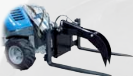
Hydraulic clamp for pallet fork
