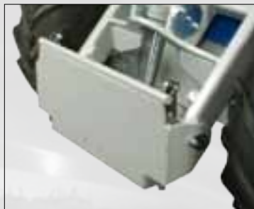
Automatic attachment coupling plate
