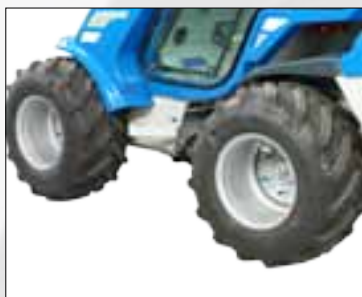
Hi torque wheel motors
